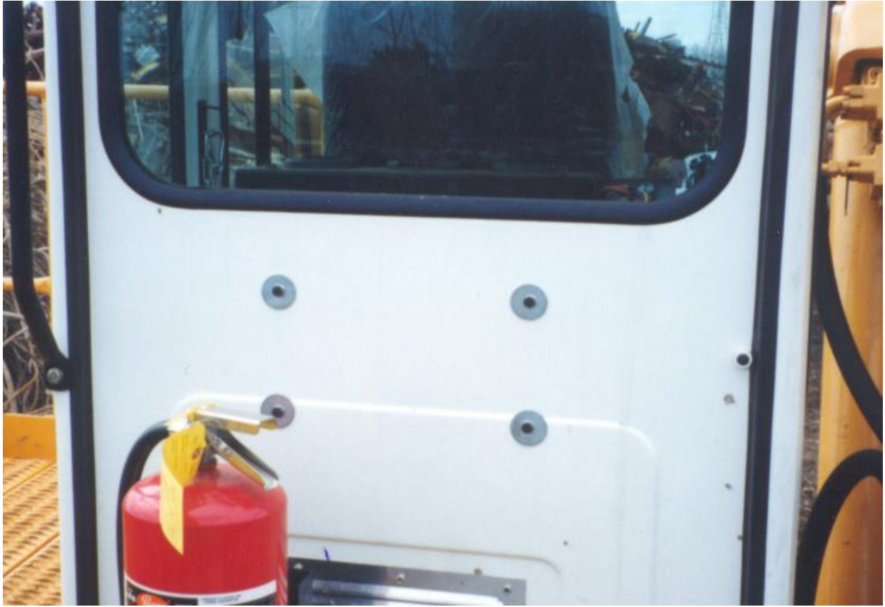
Back of cab showing mounting arrangement for evaporator.
